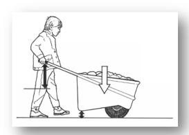
If the load is 300N and the effort required to lift it is 100N then the mechanical advantage is: 300/100 = 3/1 or 3:1 or 3
